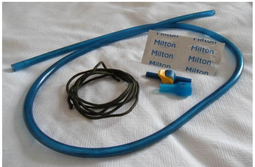
Hoses collect dirt as time goes by, not only on the outside but also inside. That mud, grease or dirt will clog up the hose in addition to making it look disgusting. Get your paracord, tie granny knots in it and pull it through that dirty hose.
